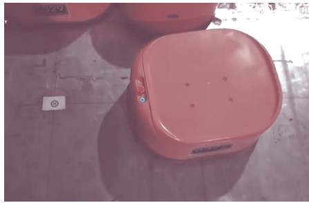
The robots at the sorting stations are able to identify the destination of a package through a code-scan, virtually eliminating sorting mistakes.
